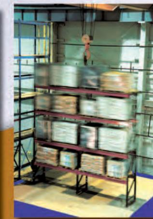
All loads remain intact on racks during the most severe earthquake simulation and structure incurs no damage!
